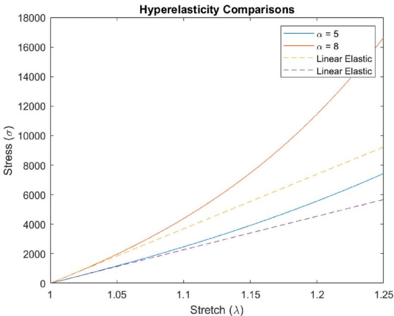
**Figure 6:** Shown above are two stress-stretch curves of hyperelastic Ogden models in uniaxial tension with corresponding linear elastic stress-stretch curves. As the stretch is increased, the hyperelastic curves demand higher stresses than the linear elastic curves. Also note that as  $\alpha$  is increased, this phenomenon is exaggerated.
