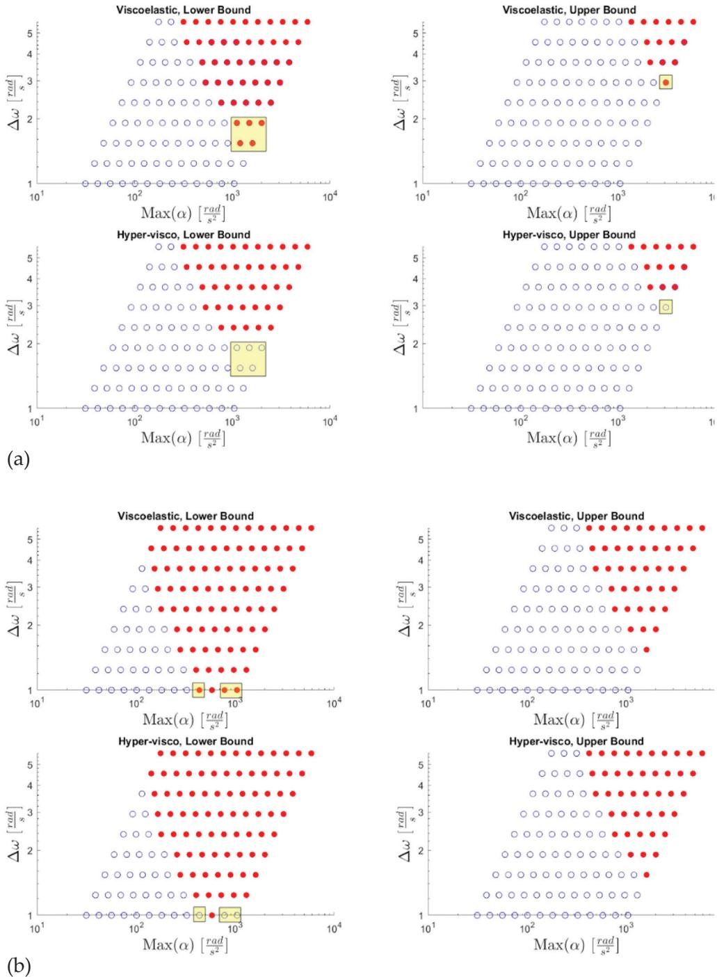
**Figure 5:** Shown above are the results of the tests given an injury condition of (a) 0.1 maximum shear strain and (b) 0.05 max shear strain. Data points in red reveal tests that recorded a maximum shear strain in the brain larger than the threshold. The differences between the viscoelastic and hyper-viscoelastic tests are highlighted in yellow.
