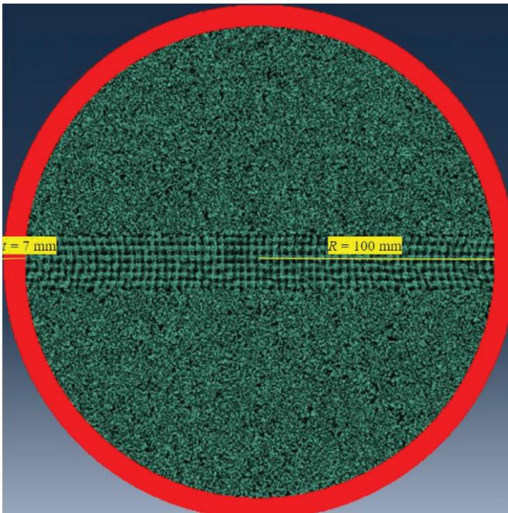
**Figure 1:** Shown above is the cross section of the *Abaqus* model brain that was used for each test. The skull is shown in red and the brain is in green. The skull is defined as a rigid body and the brain material definition varies between viscoelastic or visco-hyperelastic throughout the studies.
