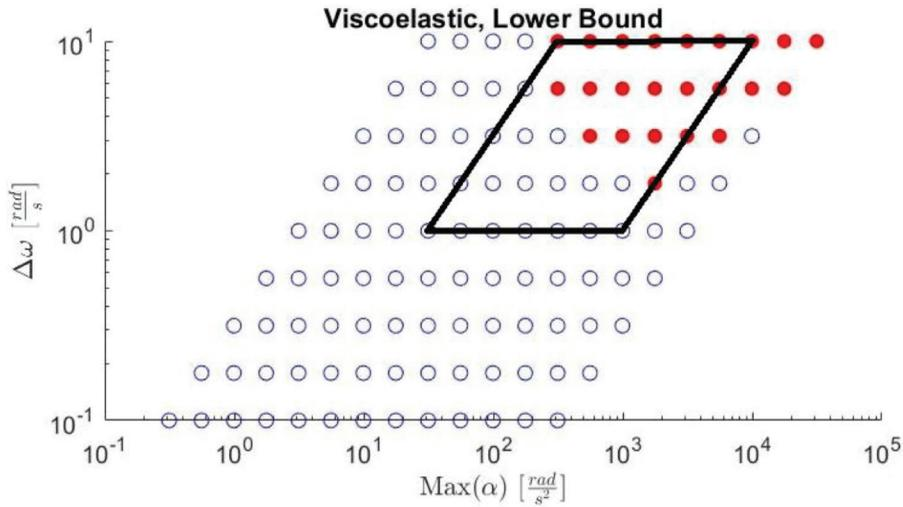
**Figure 4:** Shown above is the lower bound of the viscoelastic set of tests from the preliminary phase. The black lines show the loading input boundaries for which the second phase of tests are conducted. Notice that the two columns on the right side are excluded due to numerical dispersion, a concept that is explained in the Discussion section.
