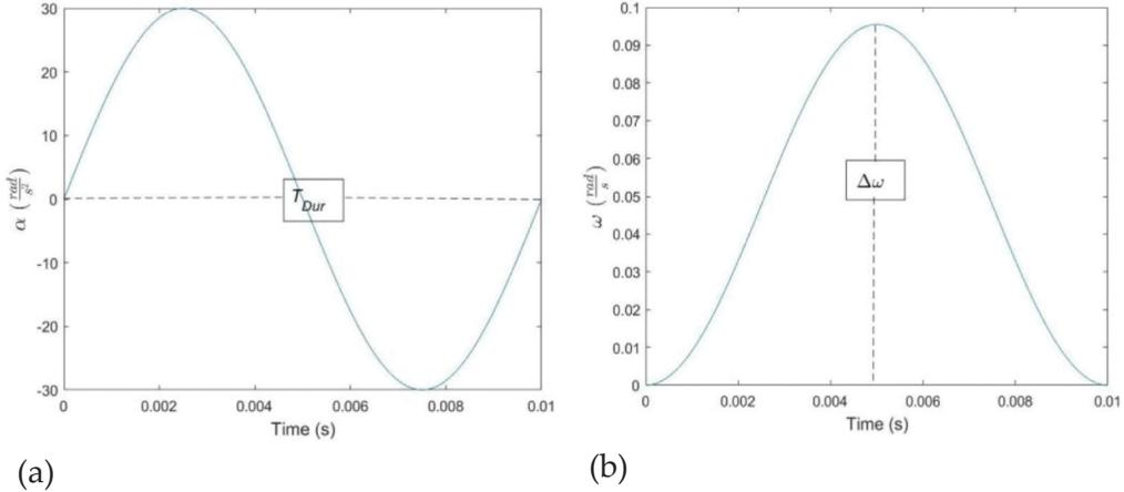
**Figure 2:** Loading specifications applied to the skull for each test. (a) The rotational acceleration delivered to the skull, with period set by  $T_{Dur}$ . (b) The rotational velocity, with magnitude set by  $\Delta\omega$ .
